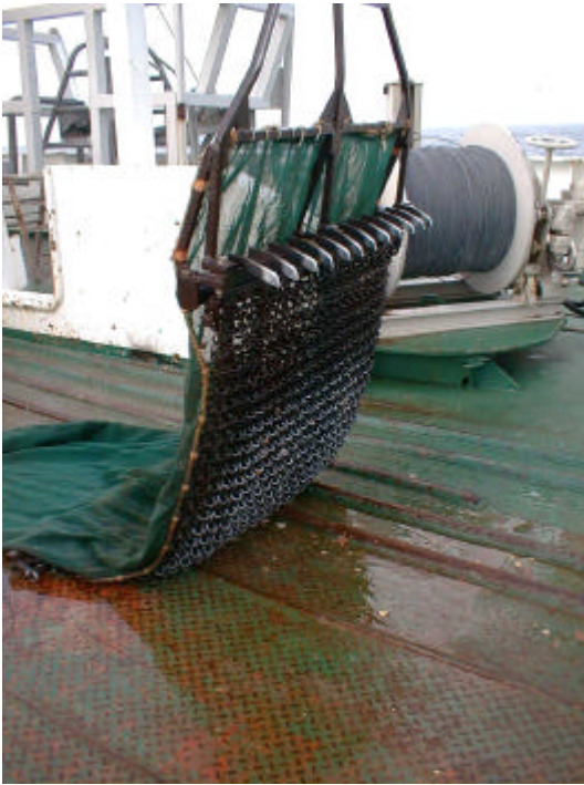
Figure 27 Modified scallop dredge used to collect samples.
